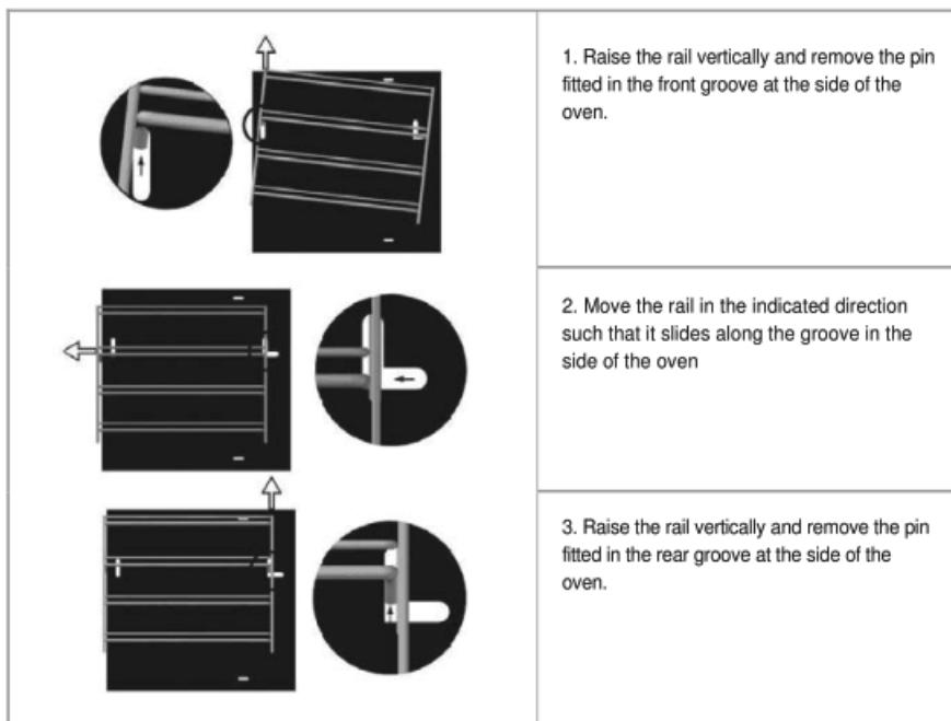
The stainless steel sliders that support the enamel roasting dishes can be removed and fitted to all three levels of side railings.
