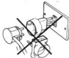
Before turning the oven on, make sure that the electrical connections and protection devices are suitable for the product's technical characteristics.
