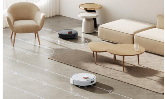
Zigzag and Y-shape cleaning routes
